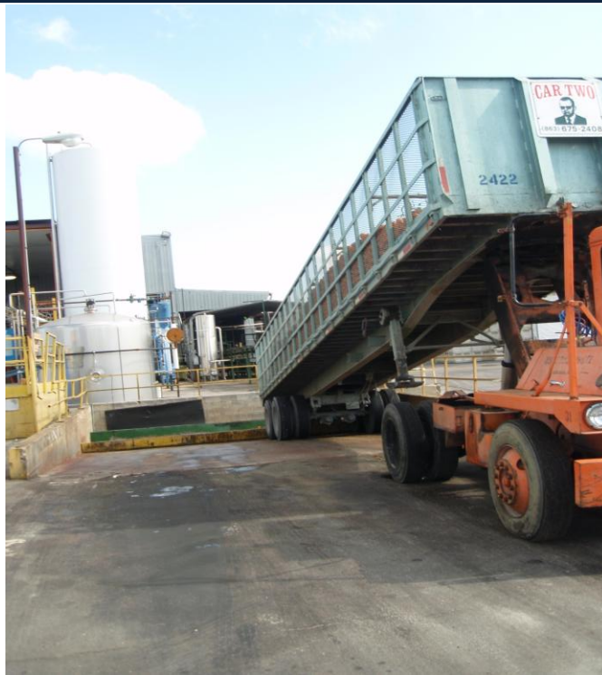
Trucks dump the citrus fruit onto a conveyor belt that takes the fruit into the juice plant (facing north).
